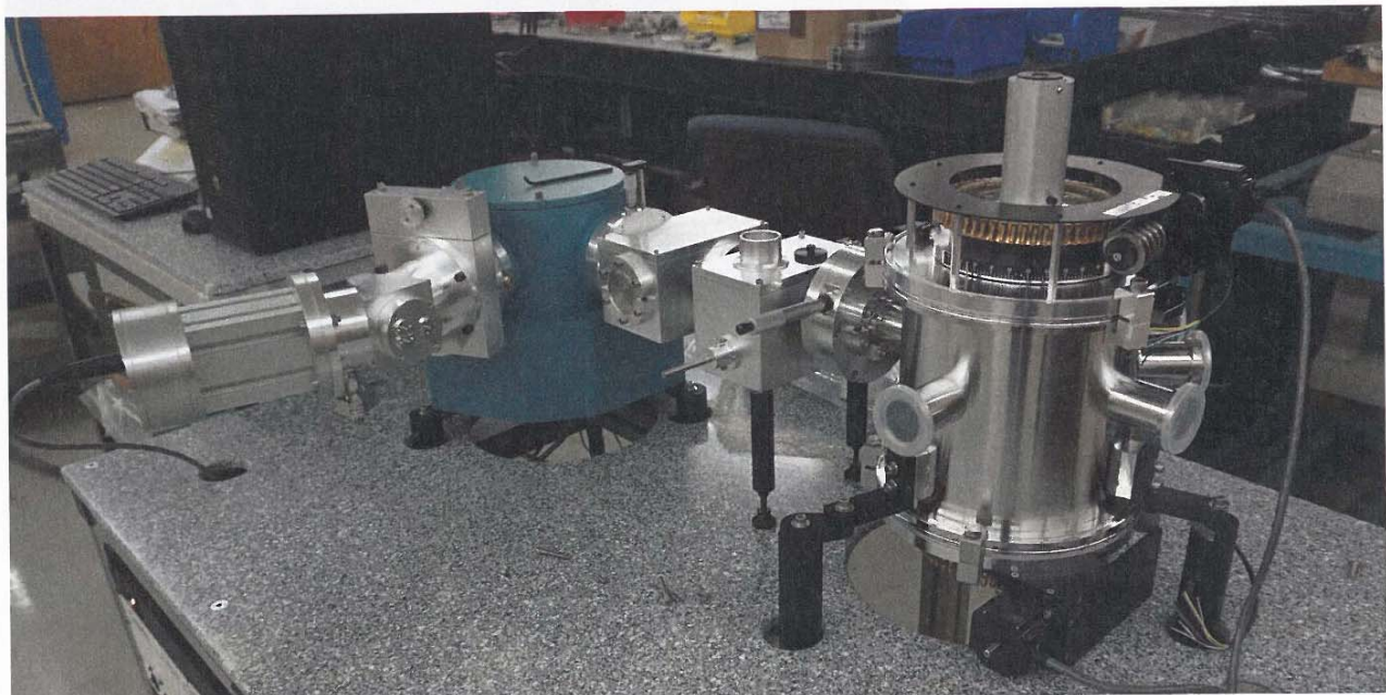
Figure 1. A vacuum- and purge-capable spectrophotometer configured as a spectral test station for measurement of plane diffraction grating efficiency and polarized response.
